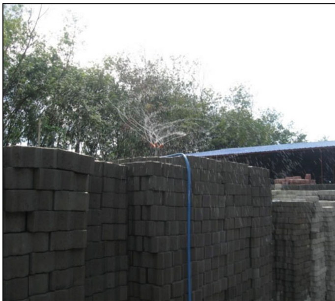
Fig. 6.10 Water curing in a block manufacturing yard
