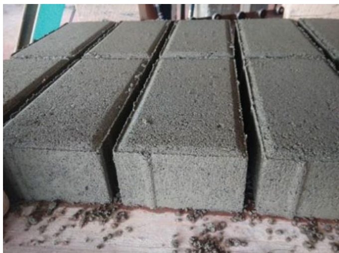
Fig. 3.6 Sample ICBP using optimized concrete mixture
