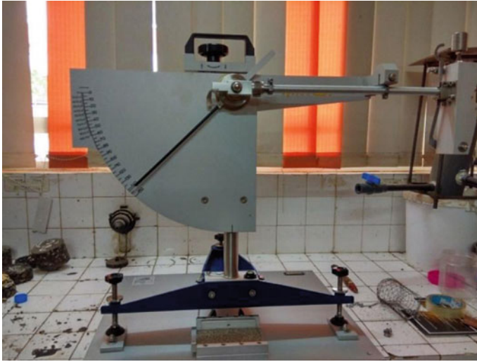
Fig. 3.3 British pendulum tester
