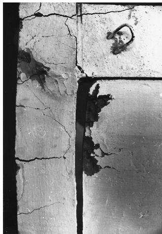
Figure 8.70 Separation of the infill from the frame; local crushing of the infill corners of frame F4R. (Adapted from Stylianidis, K. 2012. Journal of O.C.B.T. , 6, 194–212.)
