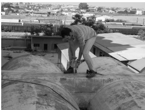
Figure 13.14 Hammer tests at MELISSARI Complex (Thessaloniki).
