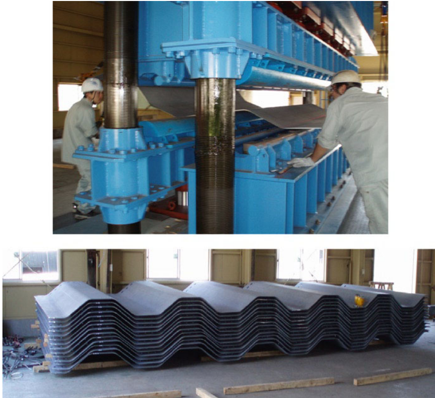
Fig. 22.17 A sophisticated press and fabricated corrugated webs
