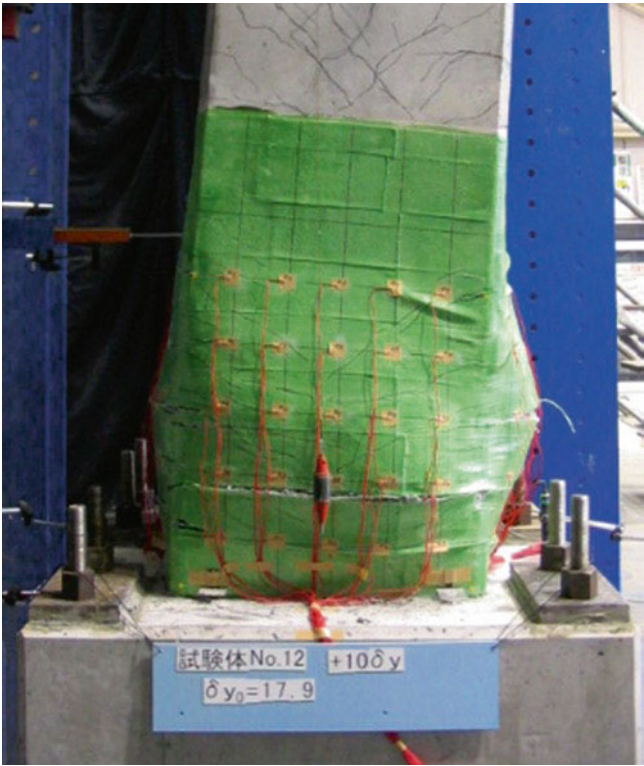
Fig. 14.6 Typical failure of RC columns jacketed with PET composites within the hinge zone at the ultimate state
