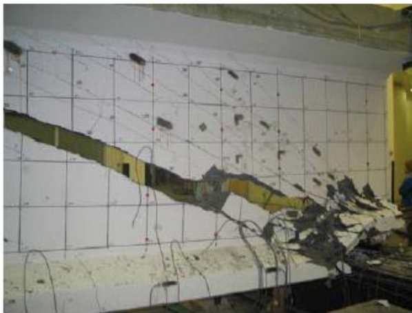
(a) Failure at East end of Girder 5
