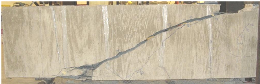
b) Regular concrete Beam B27-8 with minimum stirrup reinforcement
