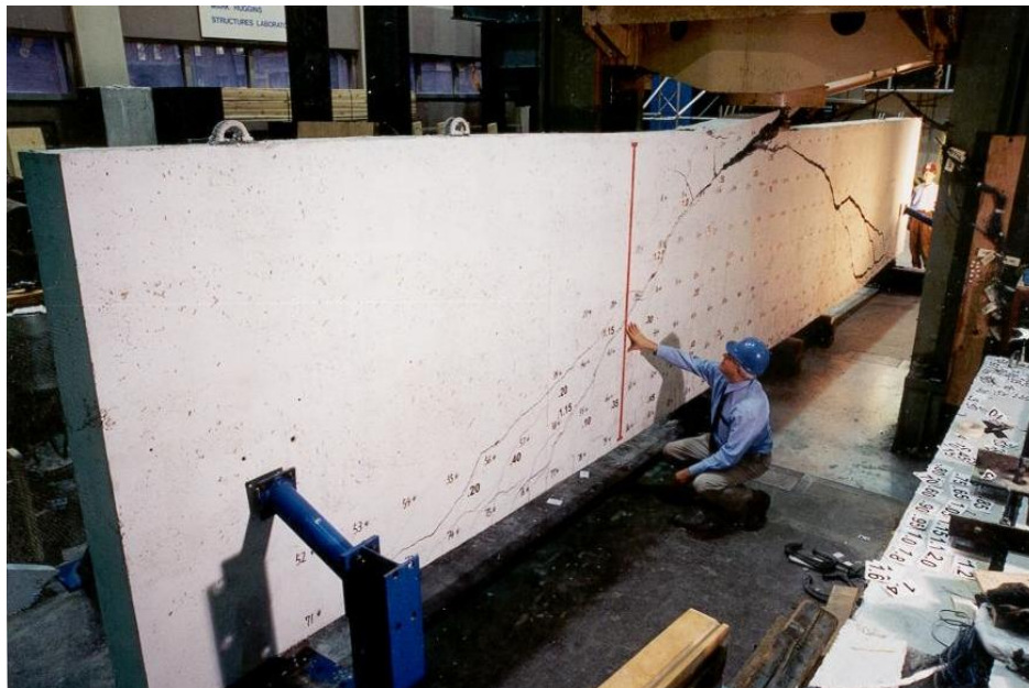
Fig. 5.11: Post-failure YB2000/9 left end with YB2000/0 on right end
