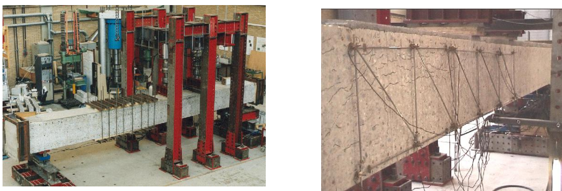
Fig. 8.6: Shear tests on beams damaged by short horizontal cracks due to alkali silica reaction (TU Delft)
