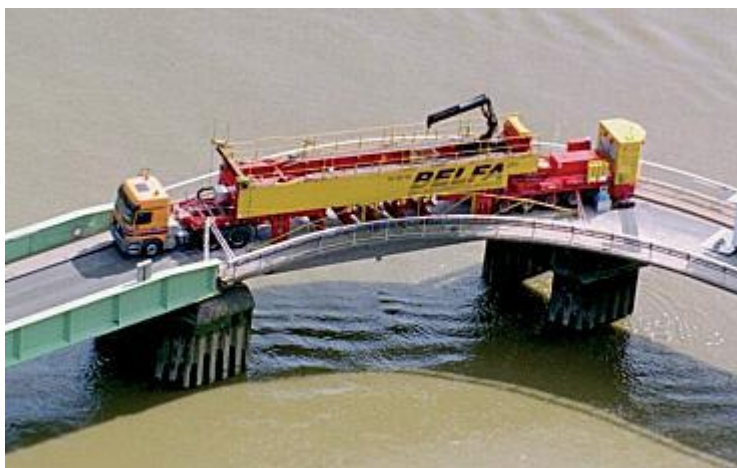
Fig. 8.11: Proof loading of an existing bridge with specially instrumented German Loading Truck (BELFA) in The Netherlands.
