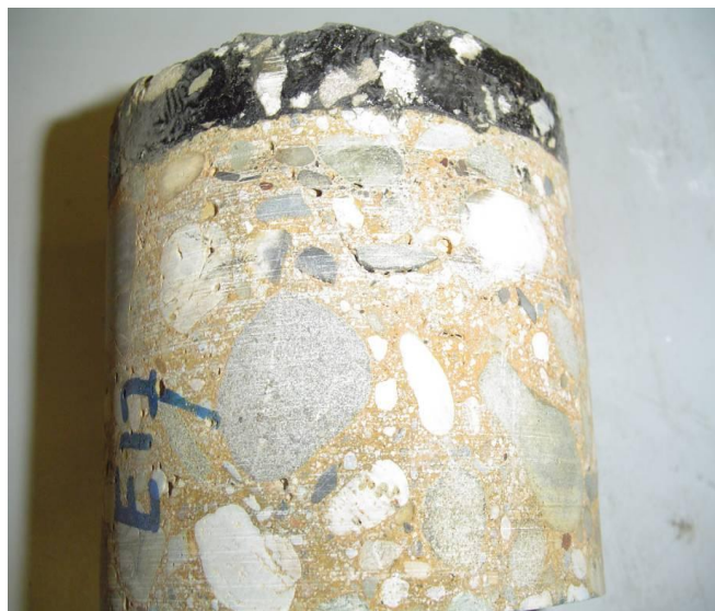
Fig. 8.5: Drilled cylinder with visual flow under one of the large particles (weakened interface)
