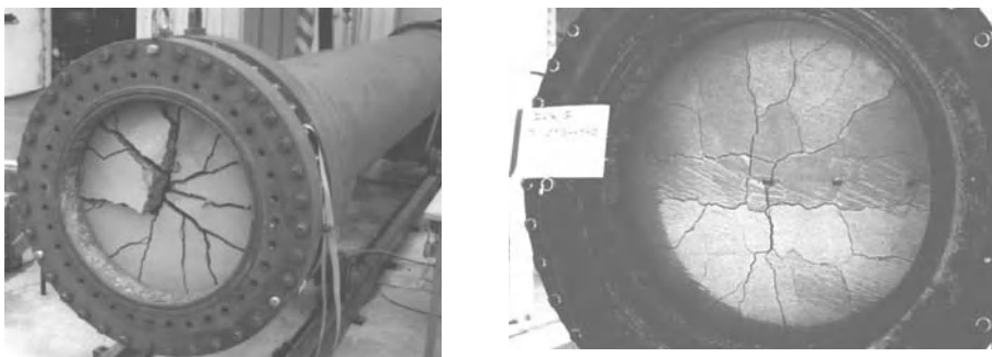
Figure 1.4. Shock tube failure trials for a plain or reinforced concrete slab (from [TOU 95a])
