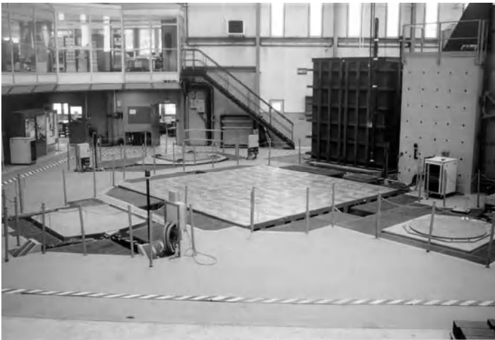
Figure 5.6. General view of the 4 shaking tables of the TAMARIS facility in Saclay
