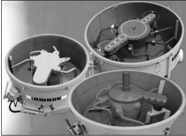
Figure 4.5 Ring-pan concrete mixers
