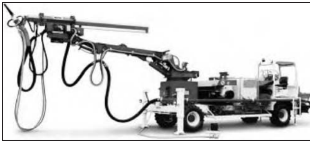
Figure 4.8 Wet-mixture shotcrete equipment with robotic nozzle
