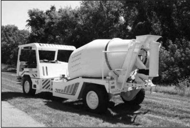
Figure 4.4 Concrete drum mixer specifically designed for underground application
