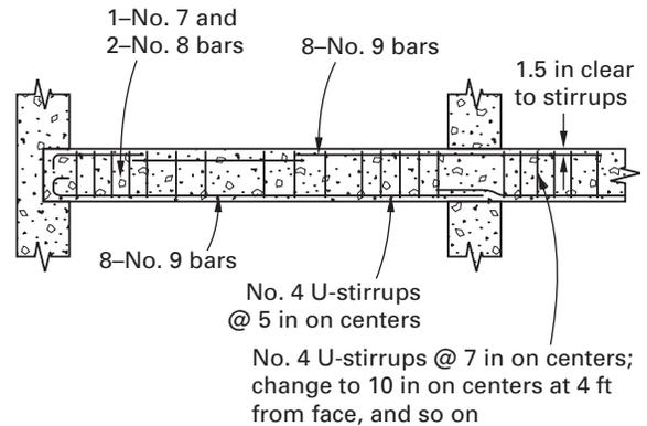
partial elevation of girders at line 1 and 2
