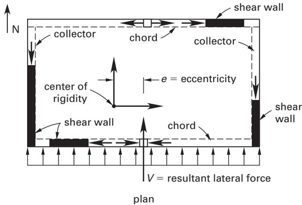
Figure 11.4 Components of a Typical Rigid Diaphragm
