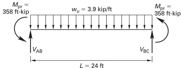
Maximum shear occurs at the left end when hinges form in the pattern shown.
