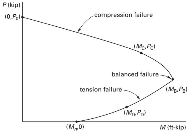
Figure 6.2 Interaction Diagram for Column of Ex. 6.2
