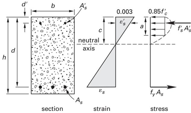
Figure 3.4 Notation for Moment Strength of a Doubly Reinforced Rectangular Beam
