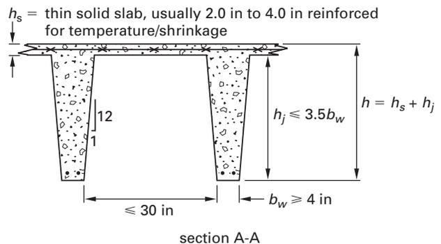
Figure 7.4 Typical One-Way Ribbed Slab System
