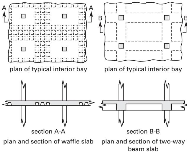
Figure 8.2 Two-Way Waffle Slab and Beam-Slab Floor Systems
