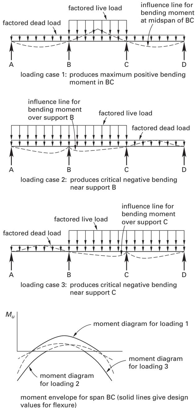
Figure 7.2 Moment Envelope for a Three-Span Continuous Beam
