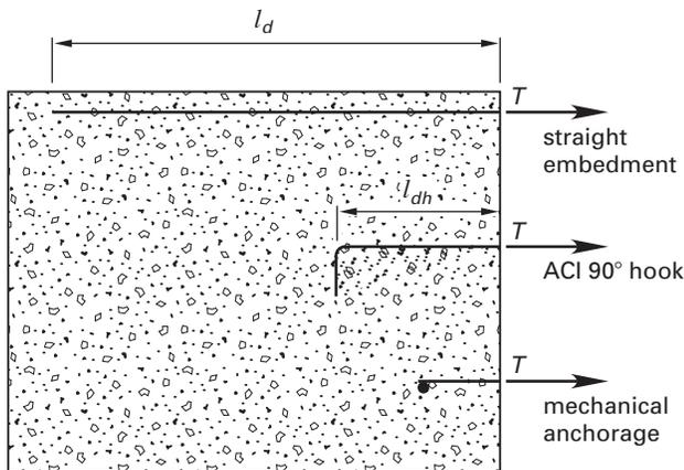
Figure 9.1 Representative Methods to Develop Bars in Tension
