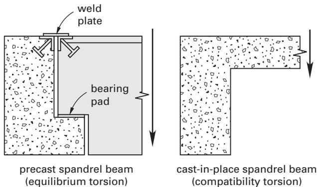
Figure 5.4 Sections Through Precast and Cast-in-Place Spandrel Beams
