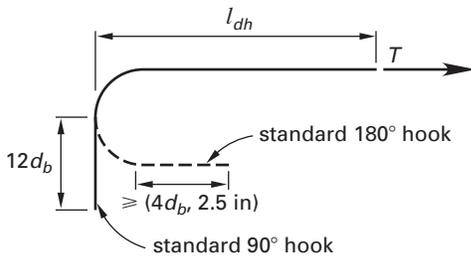
Figure 9.2 Development Length for Standard Hooks in Tension
