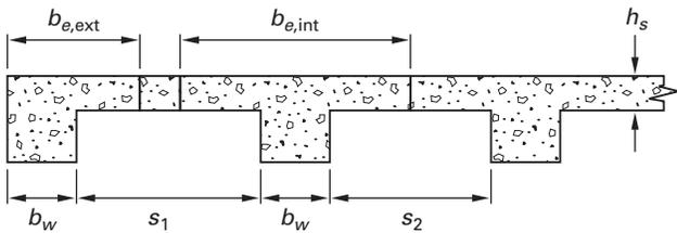
Figure 3.3 Effective Widths of T-Beams and L-Beams
