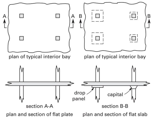
Figure 8.1 Representative Two-Way Reinforced Concrete Floor Systems
