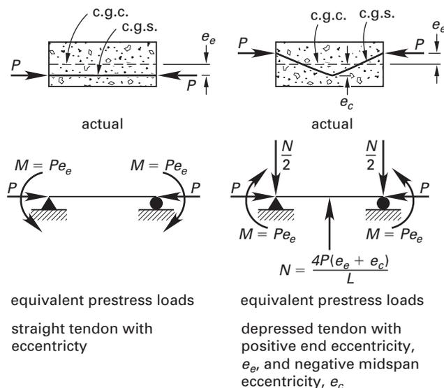
Figure 10.3 Equivalent Prestress Loads for Two Tendon Profiles
