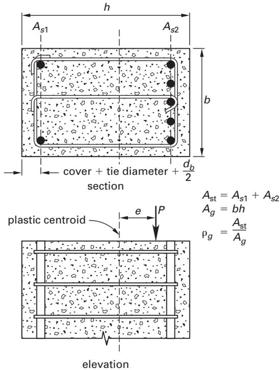
Figure 6.1 Notation for a Rectangular Reinforced Concrete Column
