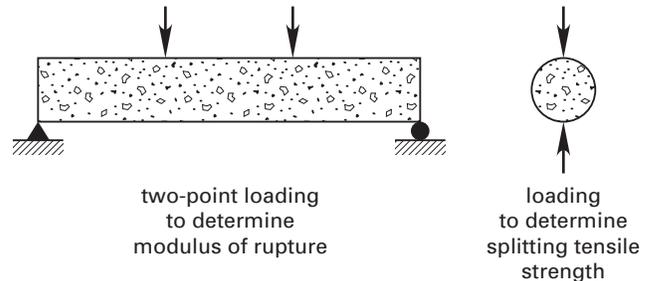
Figure 1.2 Test Arrangements to Determine Concrete Tensile Strength
