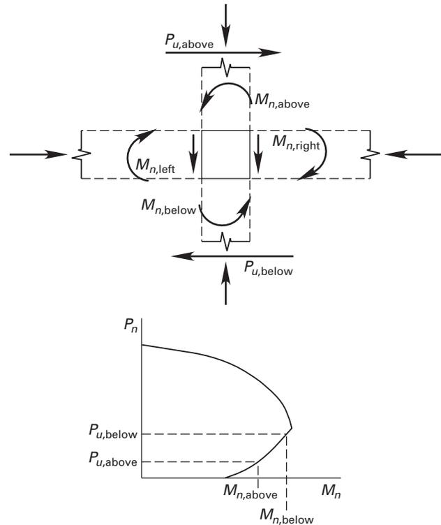
Figure 11.1 Definition of Moments Acting at Joint Faces of Special Moment Frame
