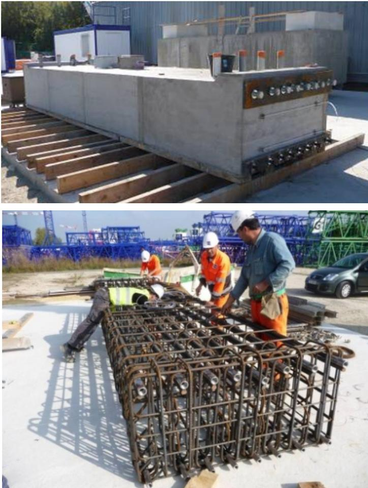
**Figure 1.1.** *RL block with free deformations (Top) and its reinforcement (Bottom)*
