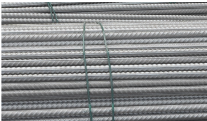
Fig. 10.3 Stainless steel reinforcing bars
