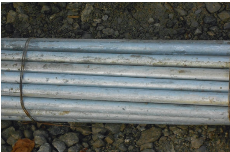
Fig. 10.4 Galvanised steel reinforcing bars
